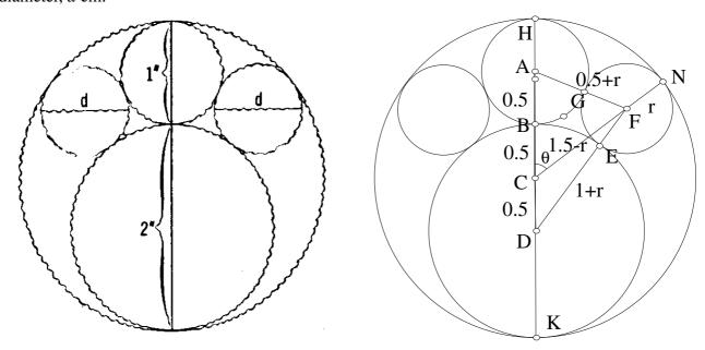
Let A be the centre of the 1 cm plug, D be the 2 cm plug, C be the 3 cm hole. Then A, C, D are collinear. Join A, C and D and produce the line segment to two ends of the diameter HK.
