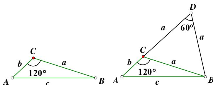
So, if  $(a, b, c)$  is a solution to a 120° triangle, then  $(a, a+b, c)$  or  $(a+b, b, c)$  is a solution to a 60° Δ.
